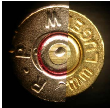
Figure 5 – Same firearm two different rounds fired (Same Breech Face Marks)
