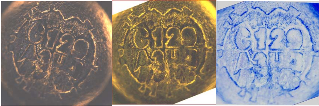
Figure 10 – gear code and multi-hit alpha numeric code (C129 / A3HJ) Images (Simple image enhancement techniques used to improved code extraction)
